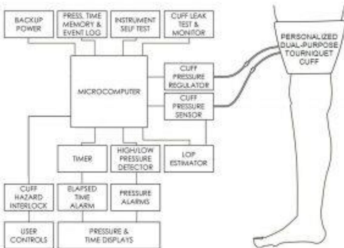
Figure 2: Modern surgical-grade tourniquet instrument and cuff adapted for BFR rehabilitation, showing elements that provide improved safety, accuracy and reliability to consistently achieve optimal patient outcomes.
